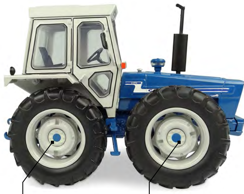
Wheel weights are fitted as standard on County 1174 to obtain maximum tractive.
